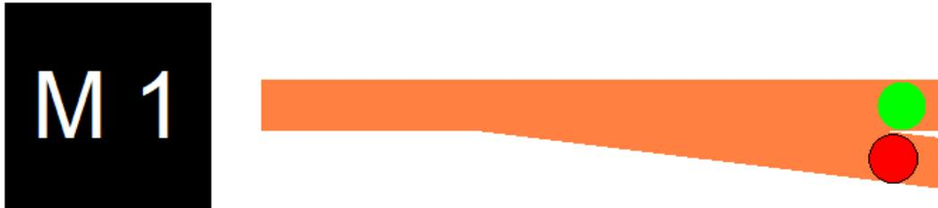
**Step 7:** Switch to the Control Panel mode. As you toggle the turnout by clicking on the red circle with the left mouse button, the motor should move from one side to the other.
