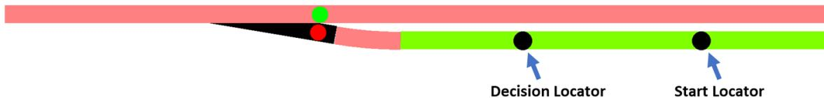
the decision locator should be placed far enough from the end of the block so that the train does not coast into the next powered block. In this case, the decision locator should be placed far enough from the end of the green control block to ensure the train stops before reaching the powered red block.
