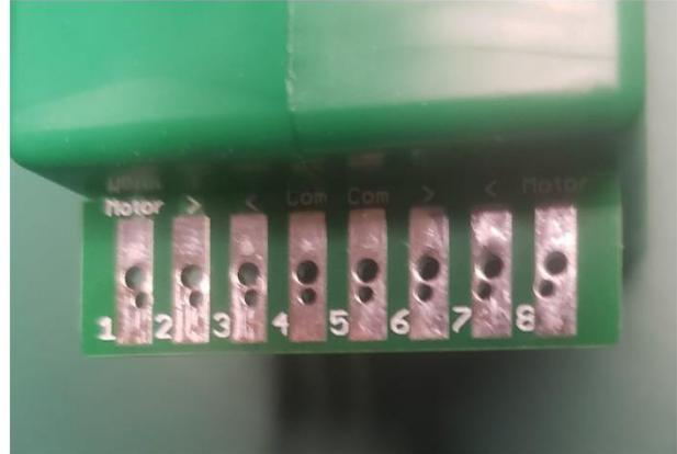
The new boards feature an industry-standard edge connector, whereas the old boards have undersized connectors and should not be used with our optional edge connector. Instead, they should be connected by soldering.
