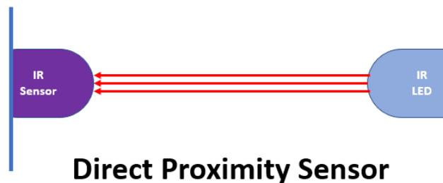
On a model railroad, the direct method can be used on opposite sides of a track to detect trains.
