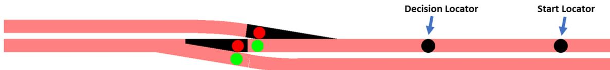
first image, a derailment situation would occur, and power should be cut. However, if the turnouts are aligned as shown in the second image, no derailment would occur, and power should not be cut. To address this, the use of a second turnout during control panel setup can be considered, which will be discussed later.
